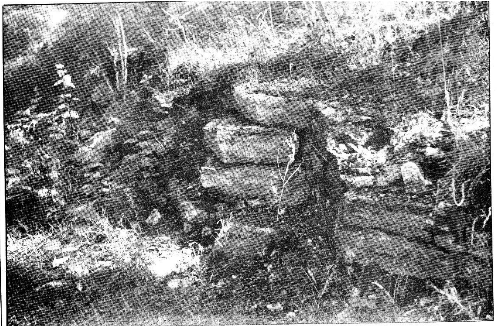
Those who have studied the geology of the Westmeath area say the condition of this limestone in a rock cut along the River Road is indicative of the type of bedrock found in candidate areas proposed for a landfill site.
